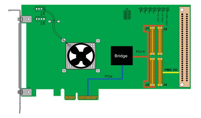
FIGURE 1. PCI104 Functional Block Diagram
